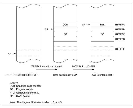
Figure 4-5 Operation when SP Value is Odd www.DataSheet4U.com
