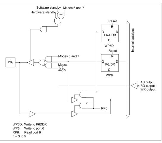
Figure C-5 (b) Port 6 Block Diagram (Pins P6<sub>3</sub> to P6<sub>5</sub>)
