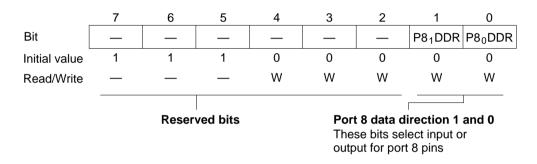
P8DDR is initialized to H'E0 by a reset and in hardware standby mode. In software standby mode it retains its previous setting. If a P8DDR bit is set to 1, the corresponding pin maintains its output state in software standby mode.
