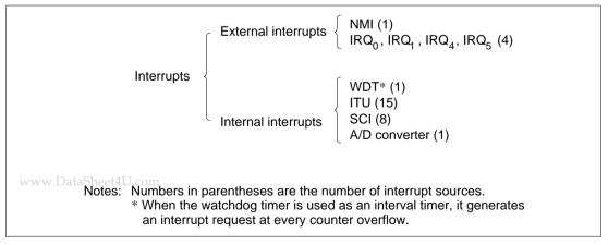
Figure 4-3 Interrupt Sources and Number of Interrupts
