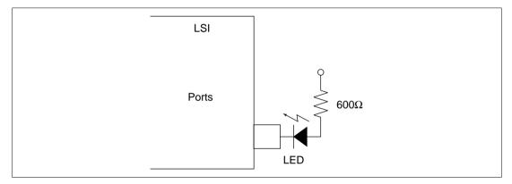
Figure 18-2 LED Drive Circuit (Example)
