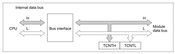
Figure 8-8 Access to Timer Counter (CPU Writes to TCNT, Upper Byte)
