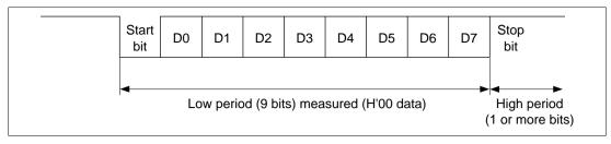
Figure 15-7 Measuring the low period of the communication data from the host
