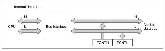
Figure 8-7 Access to Timer Counter (CPU Reads TCNT, Word)
