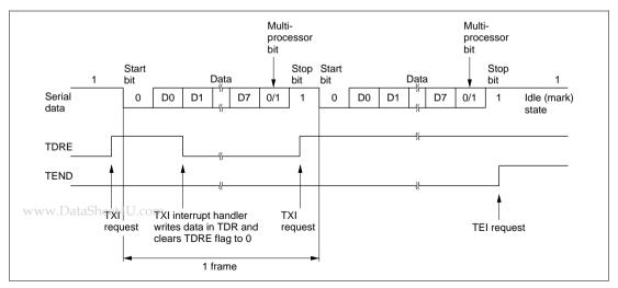
Figure 11-11 Example of SCI Transmit Operation (8-Bit Data with Multiprocessor Bit and One Stop Bit)
