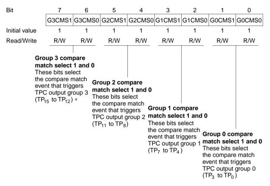
Note: \* Since this LSI does not have a TP<sub>14</sub> pin, the TP<sub>14</sub> signal cannot be output to the outside.
