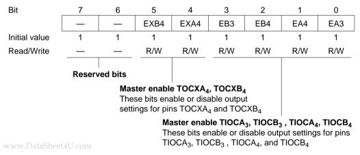
TOER is initialized to H'FF by a reset and in standby mode.
