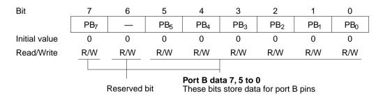
When a bit in PBDDR is set to 1, if port B is read the value of the corresponding PBDR bit is returned directly. When a bit in PBDDR is cleared to 0, if port B is read the corresponding pin level is read. Bit 6 is reserved. Bit 6 can be written and read, but cannot be used for a port input or output.
