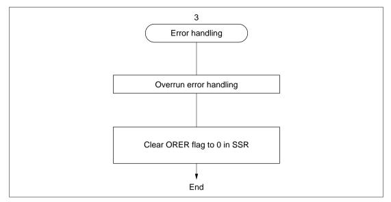
Figure 11-18 Sample Flowchart for Serial Receiving (2)
