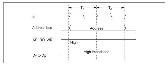
Figure 2-16 Pin States during On-Chip Memory Access
