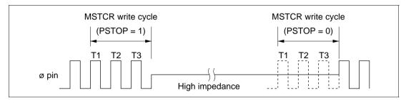
Figure 17-3 Starting and Stopping of System Clock Output
