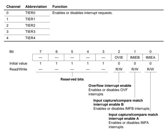
Each TIER is an 8-bit readable/writable register that enables and disables overflow interrupt requests and general register compare match and input capture interrupt requests.
