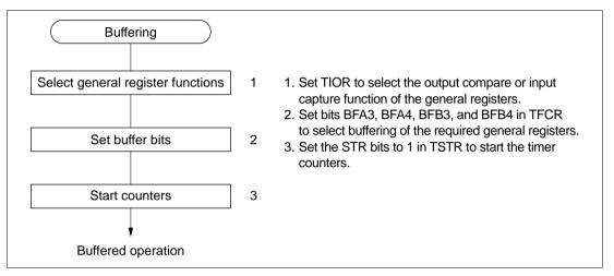
Figure 8-48 Buffering Setup Procedure (Example)
