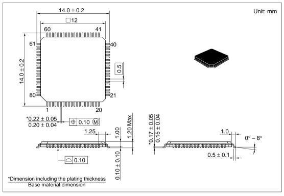
Figure G-2 Package Dimensions (TFP-80C)
