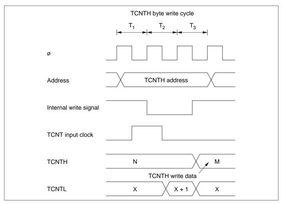
Figure 8-63 Contention between TCNT Byte Write and Increment
