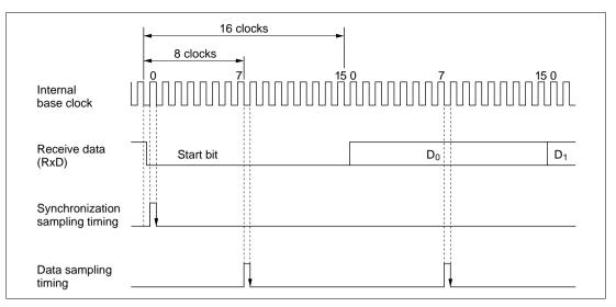
Figure 11-21 Receive Data Sampling Timing in Asynchronous Mode
