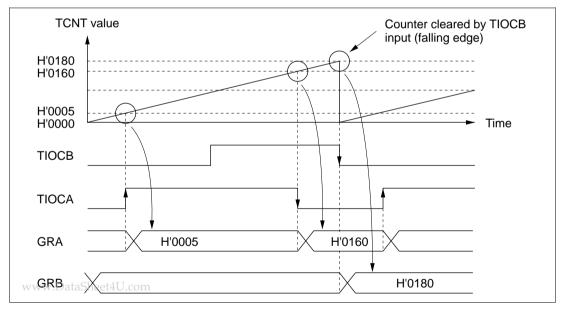
Figure 8-24 Input Capture (Example)
