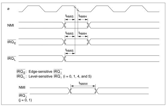
Figure 18-12 Interrupt Input Timing
