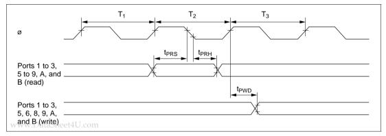
Figure 18-14 TPC and I/O Port Input/Output Timing
