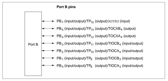
Figure 7-23 Port B Pin Configuration
