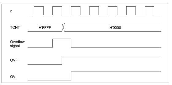
Figure 8-59 Timing of Setting of OVF
