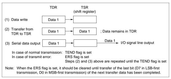
Figure 12-5 Relation Between Transmit Operation and Internal Registers
