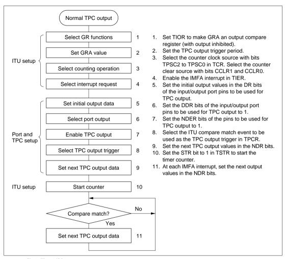
Example of Normal TPC Output (Example of Five-Phase Pulse Output): Figure 9-5 shows an example in which the TPC is used for cyclic five-phase pulse output.
