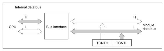
Figure 8-11 Access to Timer Counter (CPU Reads TCNT, Lower Byte)
