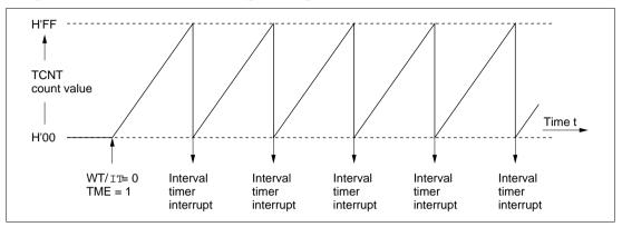
**Figure 10-5** Interval Timer Operation
