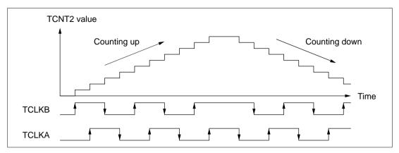
Figure 8-44 Operation in Phase Counting Mode (Example)
