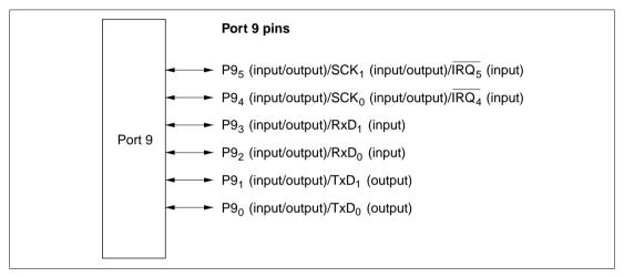
Figure 7-21 Port 9 Pin Configuration
