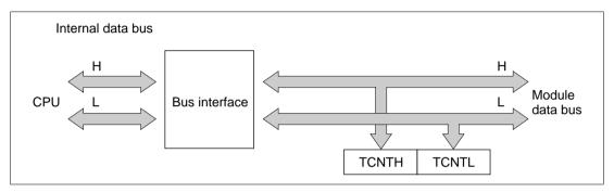
Figure 8-6 Access to Timer Counter (CPU Writes to TCNT, Word)
