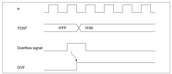
Figure 10-6 Timing of Setting of OVF
