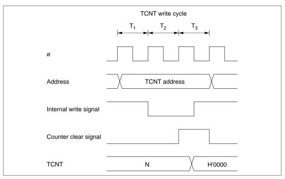
Figure 8-61 Contention between TCNT Write and Clear
