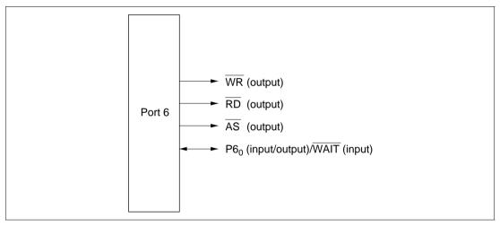
Figure 7-17 Pin Functions in Modes 1, 3, and 5 (Port 6)
