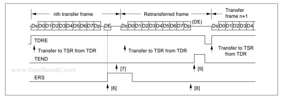
Figure 12-9 Retransfer Operation in SCI Transmit Mode
