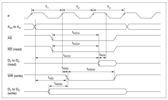
Figure 18-8 Basic Bus Cycle: Three-State Access
