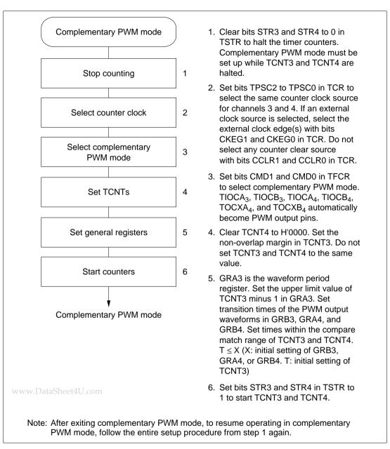
Figure 8-33 Setup Procedure for Complementary PWM Mode (Example)
