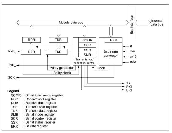
Figure 12-1 Block Diagram of Smart Card Interface
