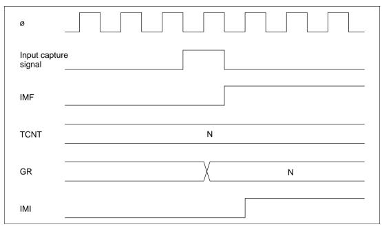
Figure 8-58 Timing of Setting of IMFA and IMFB by Input Capture
