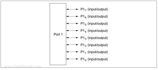
Figure 7-4 Pin Functions in Modes 6 and 7 (Port 1)
