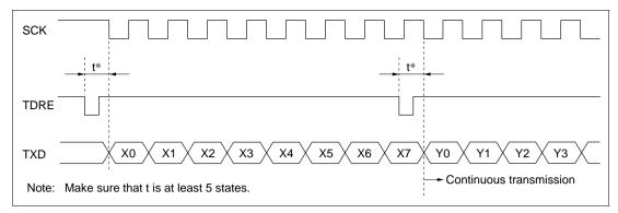
Figure 11-22 Transmission in Synchronous Mode (Example)
