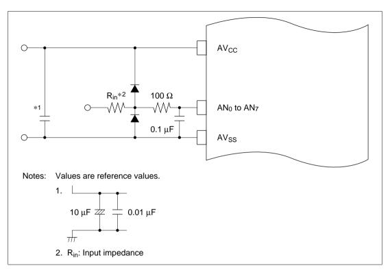
Figure 13-7 Example of Analog Input Protection Circuit
