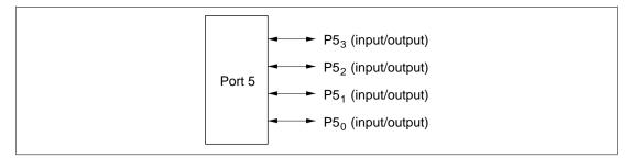
Figure 7-15 Pin Functions in Mode 6 and 7 (Port 5)
