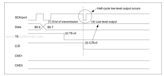
Figure 11-23 Operation when Switching from SCK Pin Functionwww.Data5hEet4tticom
