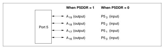
Figure 7-14 Pin Functions in Mode 5 (Port 5)
