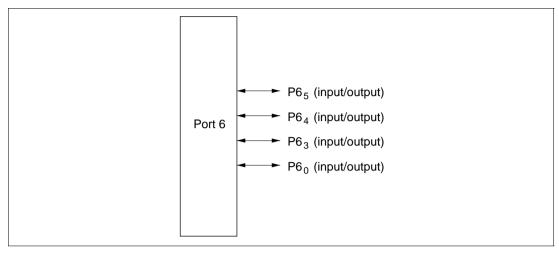
Figure 7-18 Pin Functions in Modes 6 and 7 (Port 6)
