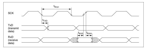
Figure 18-18 SCI Input/Output Timing in Synchronous Mode
