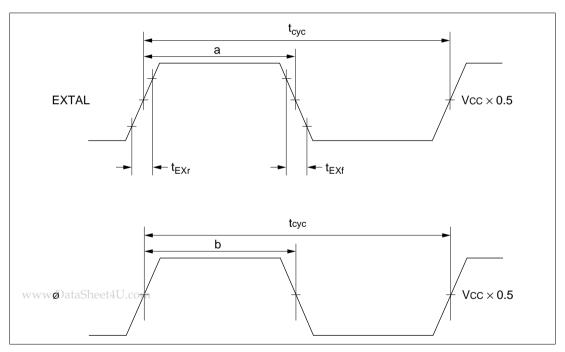
Figure 16-6 External Clock Input Timing
