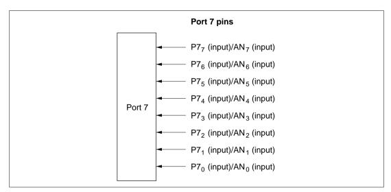
Figure 7-19 Port 7 Pin Configuration
