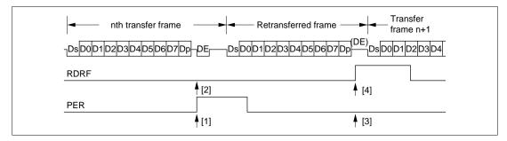
Figure 12-8 Retransfer Operation in SCI Receive Mode
