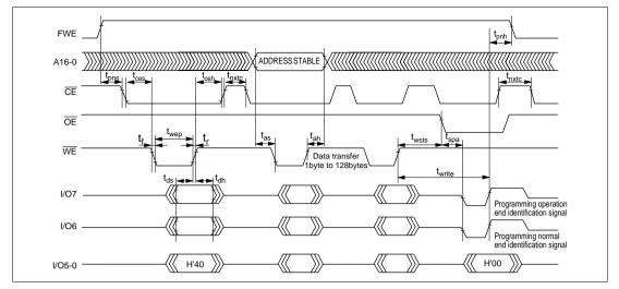
Figure 15-20 Auto-Program Mode Timing Waveforms
