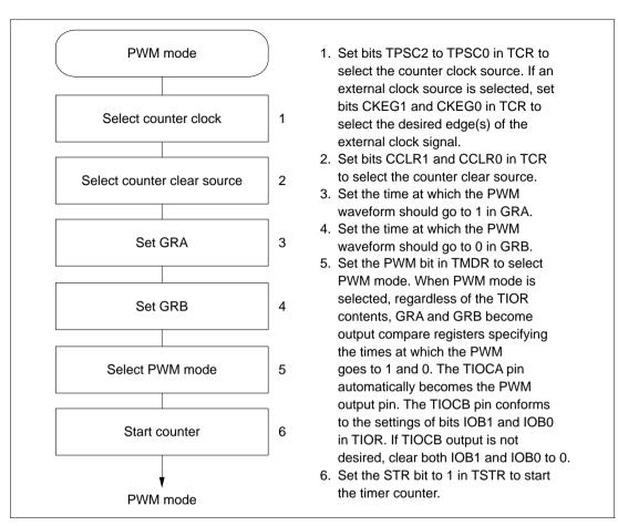
Figure 8-28 Setup Procedure for PWM Mode (Example)
