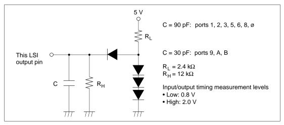
Figure 18-3 Output Load Circuit
