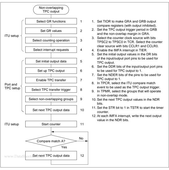
Figure 9-6 Setup Procedure for Non-Overlapping TPC Output (Example)
