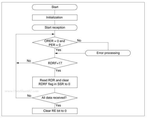
Figure 12-6 Example of Reception Processing Flow
