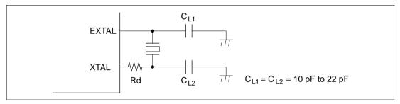
Figure 16-2 Connection of Crystal Resonator (Example)
