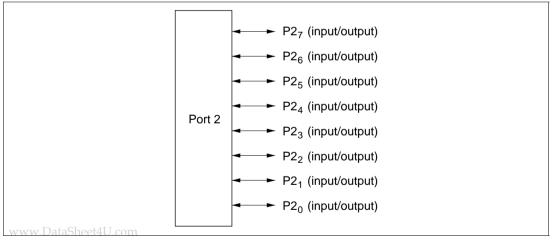
Figure 7-8 Pin Functions in Modes 6 and 7 (Port 2)
