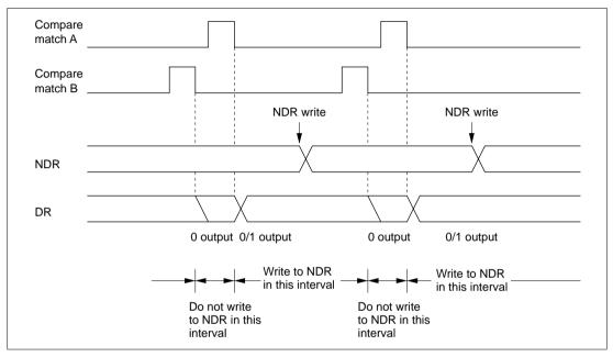
Figure 9-10 Non-Overlapping Operation and NDR Write Timing
