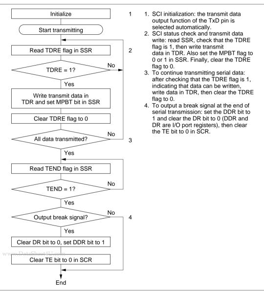
Figure 11-10 Sample Flowchart for Transmitting Multiprocessor Serial Data
