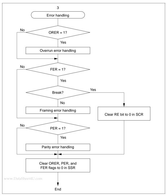
Figure 11-7 Sample Flowchart for Receiving Serial Data (2)
