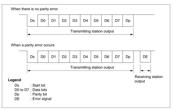
Figure 12-3 Smart Card Interface Data Format
