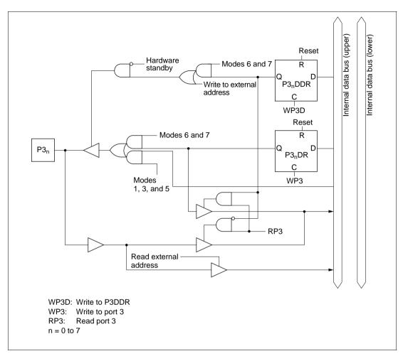
Figure C-3 Port 3 Block Diagram
