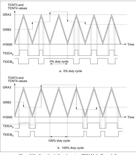
Figure 8-36 Operation in Complementary PWM Mode (Example 2) (when OLS3 = OLS4 = 1)
