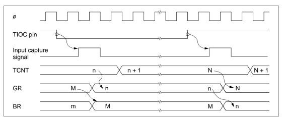
Figure 8-52 Input Capture and Buffer Transfer Timing (Example)
