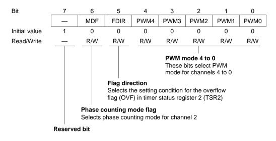
TMDR is initialized to H'80 by a reset and in standby mode.
