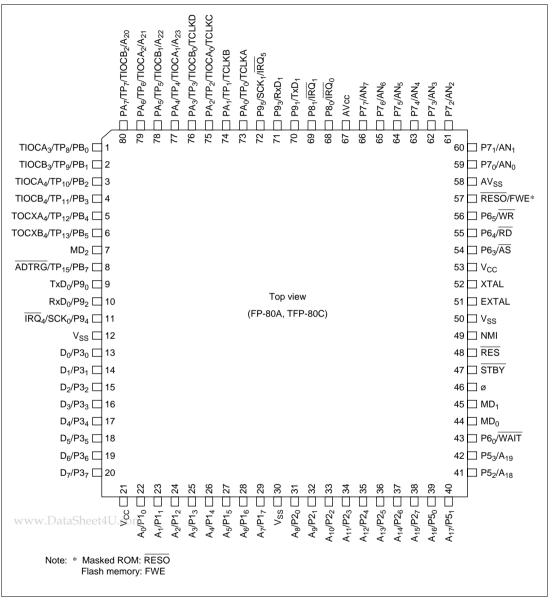
Figure 1-2 Pin Arrangement (FP-80A, TFP-80C Top View)
