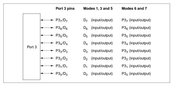
Figure 7-9 Port 3 Pin Configuration
