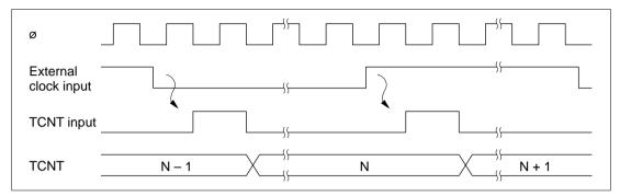
Figure 8-18 Count Timing for External Clock Sources (when Both Edges are Detected)
