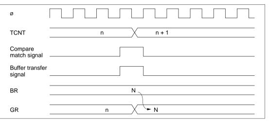
Figure 8-50 Compare Match and Buffer Transfer Timing (Example)
