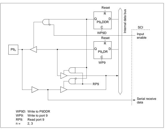
Figure C-8 (c) Port 9 Block Diagram (Pin P9<sub>2</sub>, P9<sub>3</sub>)
