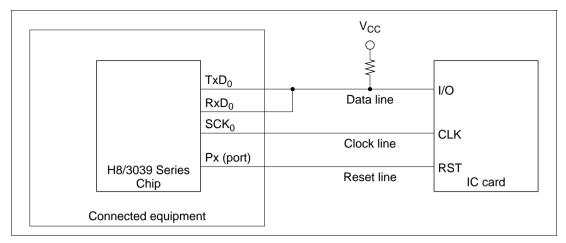
Figure 12-2 Schematic Diagram of Smart Card Interface Pin Connections
