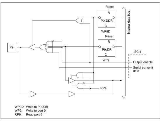
Figure C-8 (b) Port 9 Block Diagram (Pin P9<sub>1</sub>)
