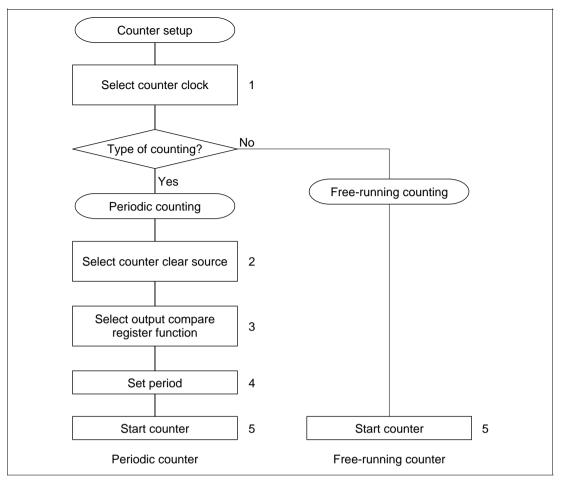
Figure 8-14 Counter Setup Procedure (Example)
