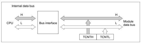
Figure 8-10 Access to Timer Counter (CPU Reads TCNT, Upper Byte)
