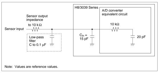
Figure 13-11 Example of Analog Input Circuit
