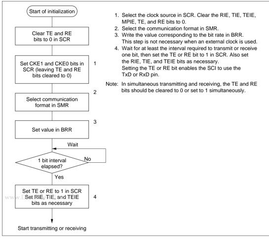
Figure 11-15 Sample Flowchart for SCI Initialization
