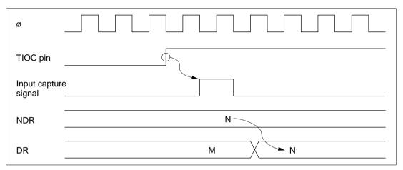
Figure 9-8 TPC Output Triggering by Input Capture (Example)
