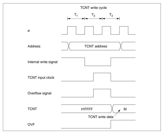
Figure 8-65 Contention between TCNT Write and Overflow
