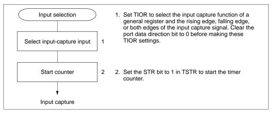
Figure 8-23 Setup Procedure for Input Capture (Example)
