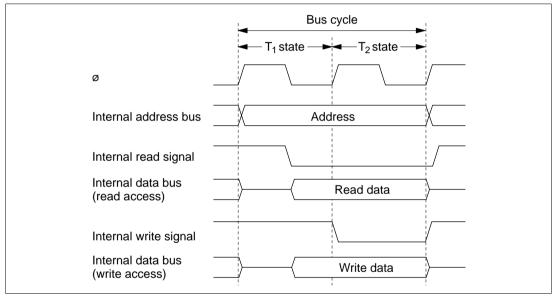
Figure 2-15 On-Chip Memory Access Cycle
