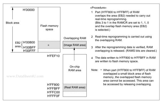
Figure 15-14 Example of RAM Overlapping Operation
