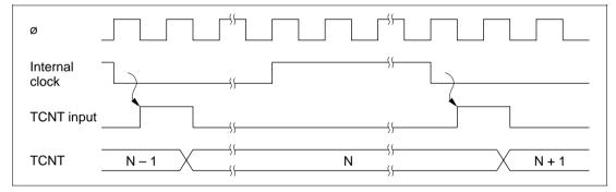
Figure 8-17 Count Timing for Internal Clock Sources
