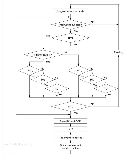
Figure 5-4 Process Up to Interrupt Acceptance when UE = 1
