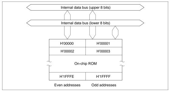
Figure 15-28 ROM Block Diagram (H8/3039)
