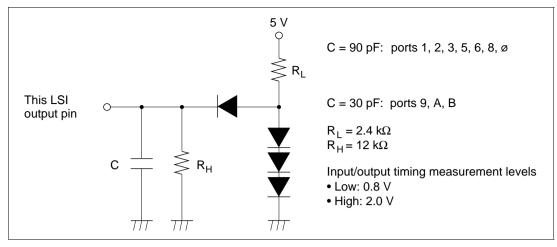
Figure 18-6 Output Load Circuit
