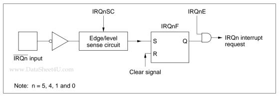
Figure 5-2 Block Diagram of Interrupts IRQ<sub>5</sub>, IRQ<sub>4</sub>, IRQ<sub>1</sub>, and IRQ<sub>0</sub>
