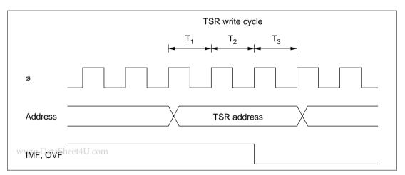
Figure 8-60 Timing of Clearing of Status Flags
