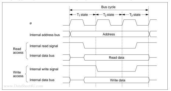
Figure 2-17 Access Cycle for On-Chip Supporting Modules
