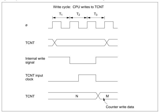
**Figure 10-8** Contention between TCNT Write and Increment Changing CKS2 to CKS0 Values: Halt TCNT by clearing the TME bit to 0 in TCSR before changing the values of bits CKS2 to CKS0.
