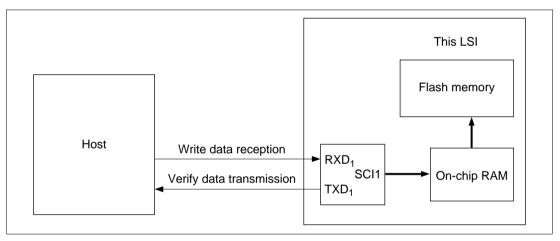
Figure 15-5 System Configuration in Boot Mode
