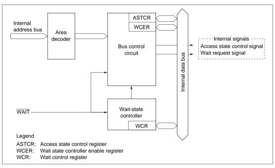
Figure 6-1 Block Diagram of Bus Controller
