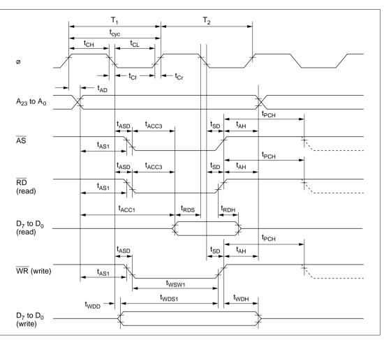
Figure 18-7 Basic Bus Cycle: Two-State Access
