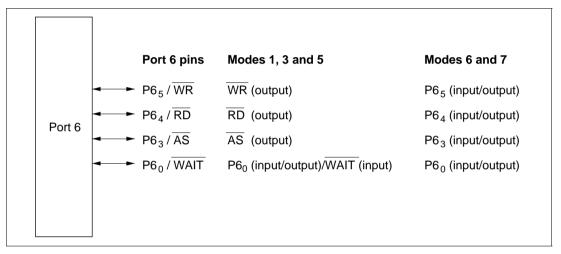
Figure 7-16 Port 6 Pin Configuration
