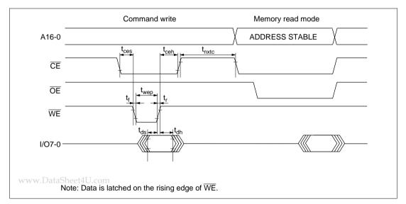
Figure 15-16 Timing Waveform in Memory Read Mode Transition
