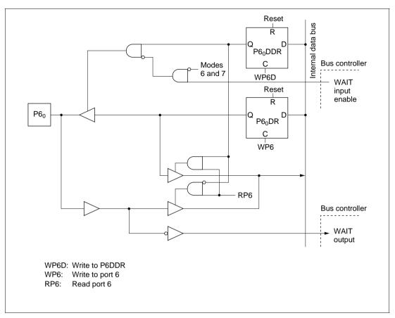
Figure C-5 (a) Port 6 Block Diagram (Pin P6<sub>0</sub>)
