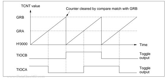
Figure 8-21 Toggle Output (Example)
