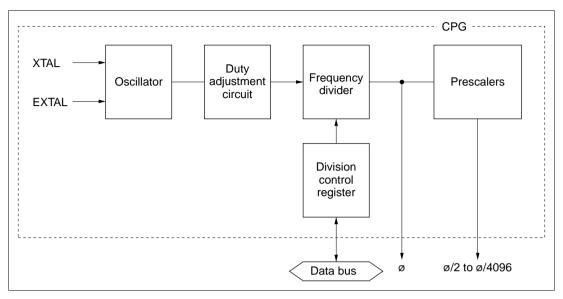
Figure 16-1 Block Diagram of Clock Pulse Generator
