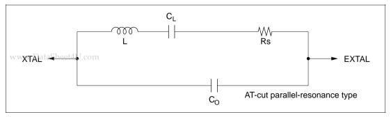
Figure 16-3 Crystal Resonator Equivalent Circuit
