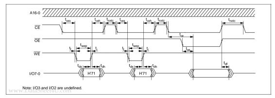
Figure 15-22 Status Read Mode Timing Waveforms
