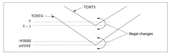
Figure 8-41 Changing a General Register Setting by Buffer Transfer (Caution 2)
