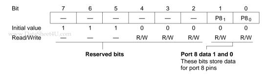
When a bit in P8DDR is set to 1, if port 8 is read the value of the corresponding P8DR bit is returned directly. When a bit in P8DDR is cleared to 0, if port 8 is read the corresponding pin level is read. www.DataSheet4U.com
