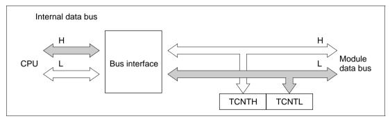
Figure 8-9 Access to Timer Counter (CPU Writes to TCNT, Lower Byte)
