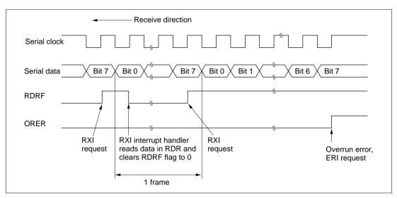
Figure 11-19 Example of SCI Receive Operation
