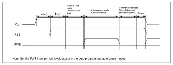
Figure 15-23 Oscillation Stabilization Time, Boot Program Transfer Time
