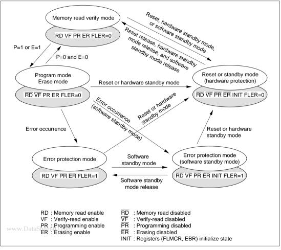
Figure 15-13 Flash Memory State Transitions (When High level apply to FWE pin in modes 5 and 7 (on-chip ROM enabled))
