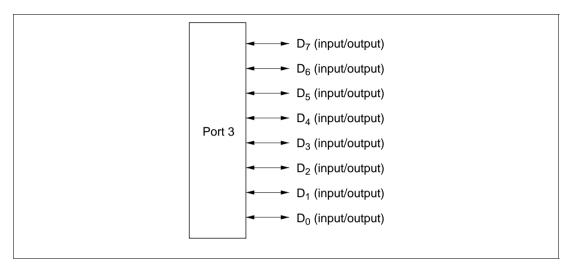
Figure 7-10 Pin Functions in Modes 1, 3 and 5 (Port 3)
