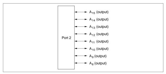
Figure 7-6 Pin Functions in Modes 1 and 3 (Port 2)
