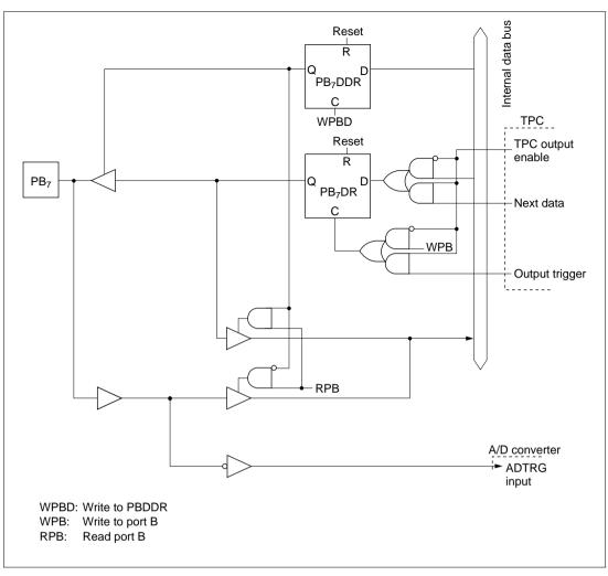
Figure C-10 (c) Port B Block Diagram (Pin PB<sub>7</sub>)
