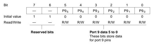
When a bit in P9DDR is set to 1, if port 9 is read the value of the corresponding P9DR bit is returned. When a bit in P9DDR is cleared to 0, if port 9 is read the corresponding pin level is read.
