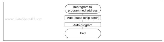
Figure 15-24 Reprogramming to Programmed Address
