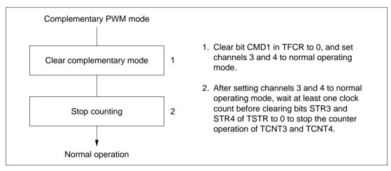
Figure 8-34 Clearing Procedure for Complementary PWM Mode (Example)
