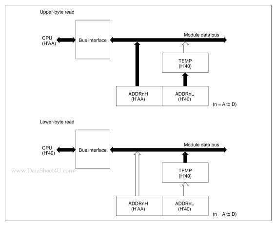
Figure 13-2 A/D Data Register Access Operation (Reading H'AA40)
