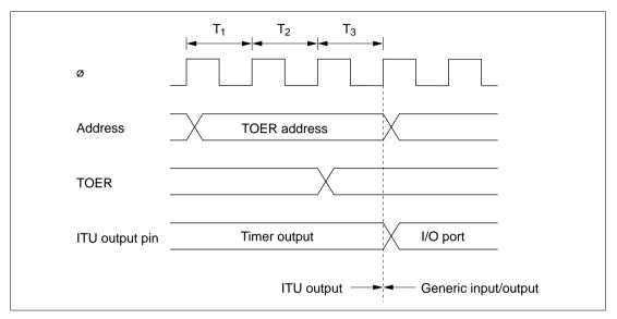
Figure 8-54 Timing of Disabling of ITU Output by Writing to TOER (Example)
