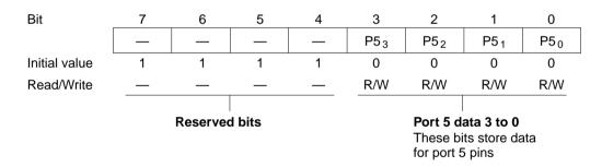
When a bit in P5DDR is set to 1, if port 5 is read the value of the corresponding P5DR bit is returned directly, regardless of the actual state of the pin. When a bit in P5DDR is cleared to 0, if port 5 is read the corresponding pin level is read.
