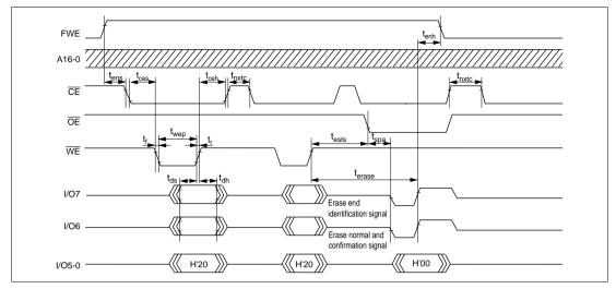
Figure 15-21 Auto-Erase Mode Timing Waveforms
