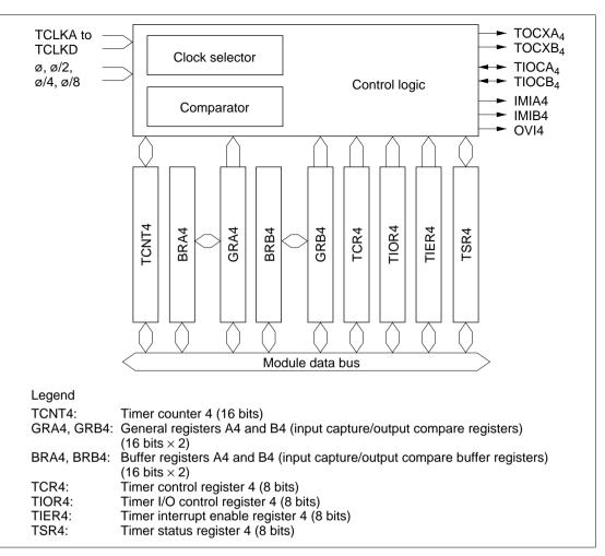
Figure 8-5 Block Diagram of Channel 4
