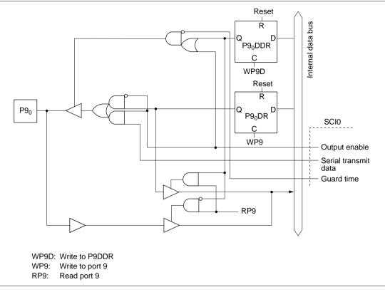
Figure C-8 (a) Port 9 Block Diagram (Pin P9<sub>0</sub>)
