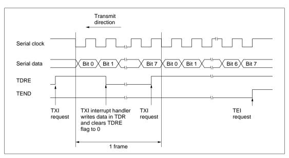
Figure 11-17 Example of SCI Transmit Operation
