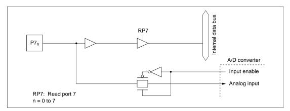
Figure C-6 Port 7 Block Diagram
