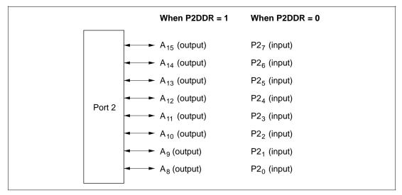
Figure 7-7 Pin Functions in Modes 1 and 3 (Port 2)
