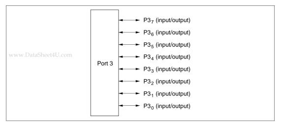
Figure 7-11 Pin Functions in Modes 6 and 7 (Portww.DataSheet4U.com
