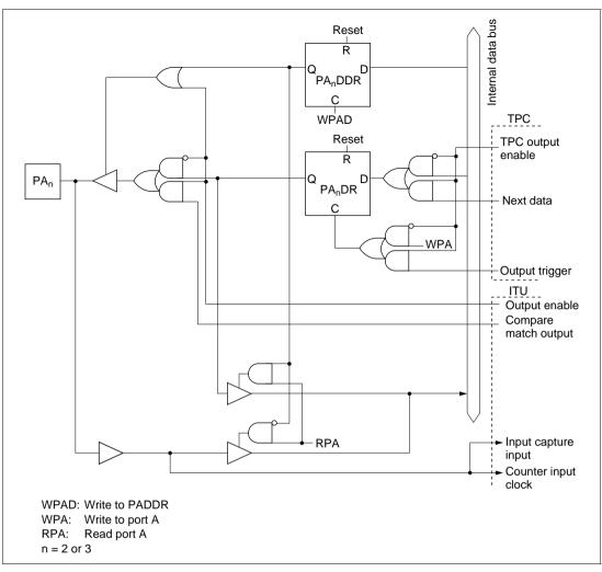
Figure C-9 (b) Port A Block Diagram (Pins PA<sub>2</sub>, PA<sub>3</sub>)
