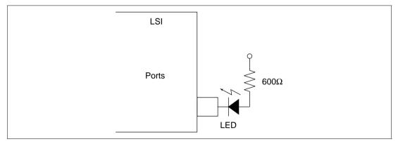
Figure 18-5 LED Drive Circuit (Example)
