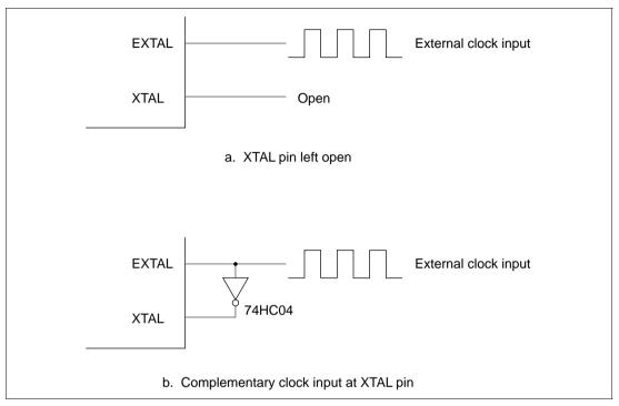
Figure 16-5 External Clock Input (Examples)
