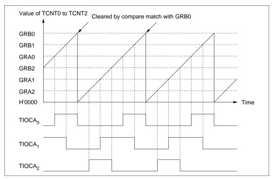
Figure 8-27 Synchronization (Example)
