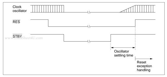
Figure 17-2 Hardware Standby Mode Timingwww.DataSheet4U.com
