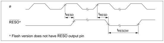
Figure 18-11 Reset Output Timing
