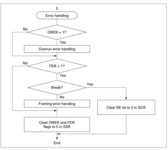
Figure 11-12 Sample Flowchart for Receiving Multiprocessor Serial Data (2)
