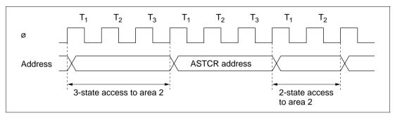
Figure 6-11 ASTCR Write Timing
