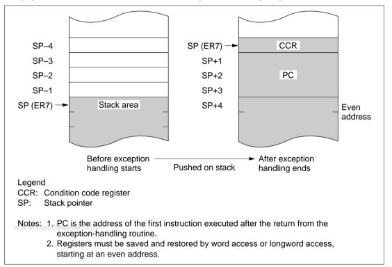
Figure 2-14 Stack Structure after Exception Handling
