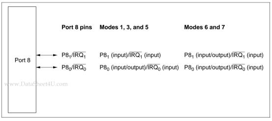
Figure 7-20 Port 8 Pin Configuration
