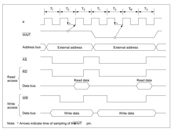
Figure 6-7 shows the timing when the wait count is 1.
