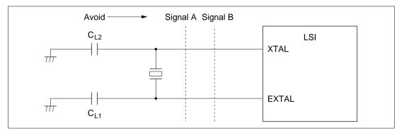
Figure 16-4 Example of Incorrect Board Design
