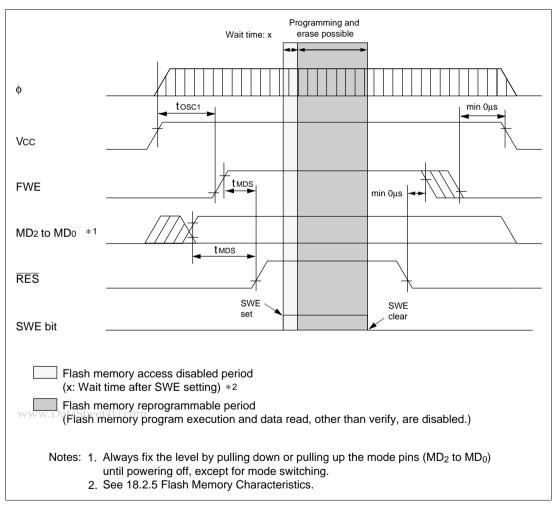
Figure 15-25 Powering On/Off Timing (Boot Mode)
