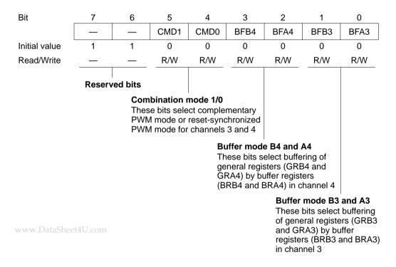
TFCR is initialized to H'C0 by a reset and in standby mode.
