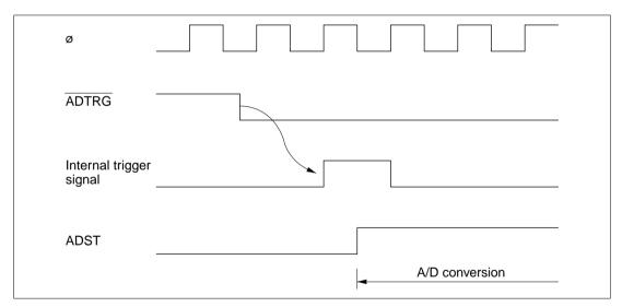
www.DataSheet4U.com Figure 13-6 External Trigger Input Timing
