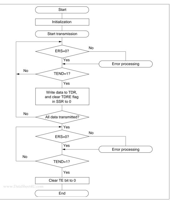
Figure 12-4 Example of Transmission Processing Flow
